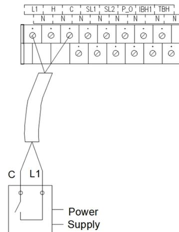
Method 3: When "Thermostat Control" is set to "Dual Zone Switching".
