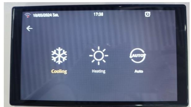
Note: Enter the password "168" in "Parameter" and set the heating & cooling type by modifying N02.
