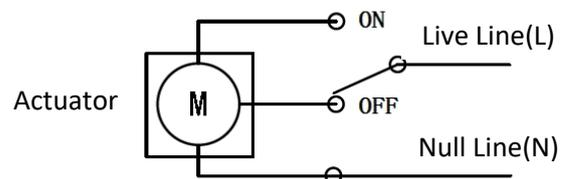
Three-way valve wiring specifications are shown in the following diagram.
