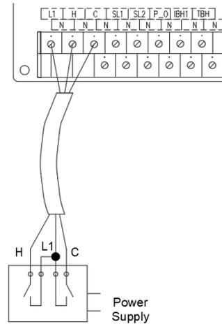
Method 2, When "Thermostat Control" is set to "Single Zone Switch".
