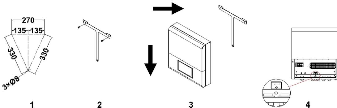
2. When the unit is mounted on the wall, the top fixing holes need to be installed in place at the same time to fix the unit when it is hung on the wall to prevent the unit from moving upwards for other reasons and thus falling off.
